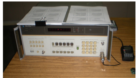
Using the precision test oscillator and the stepped attenuator to check calibration of the Ten Tec "S" meter
