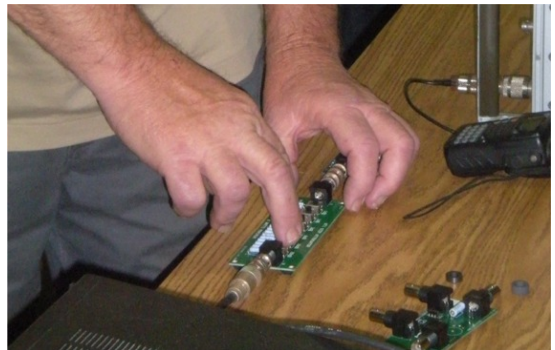
Using the precision test oscillator and the stepped attenuator to check calibration of the Ten Tec "S" meter
