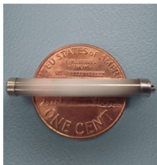
An implantable microstimulator of the kind that would be used with a wireless medical micropower network.
