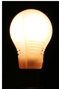
The FCC's OET said emissions from RF LED lighting devices are non-periodic, broadband in nature, and are produced as a byproduct of the internal driver circuitry within the RF LED lighting device. [Rick Lindquist, WW1ME, photo]
